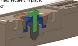
Sealing the housing can also be done in various ways: applying an adhesive on the cover or using a gasket between the housing parts are two of the most commonly used design solutions. Microprecison uses an ultrasonic welding process which does not add another material to the seal ensuring it supports the temperature requirements under UL.
